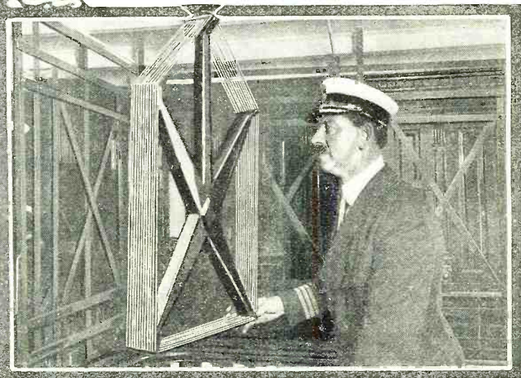
Familiar as the waters of New York Bay are to Capt. William G. Hamilton, the heavy fogs which drift over them make it often necessary to resort to the "Macom's" radio compass, as shown below.
